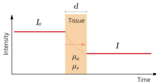
**Figure 2.4:** Continuous Wave NIRS principle, fig. taken from [11].
