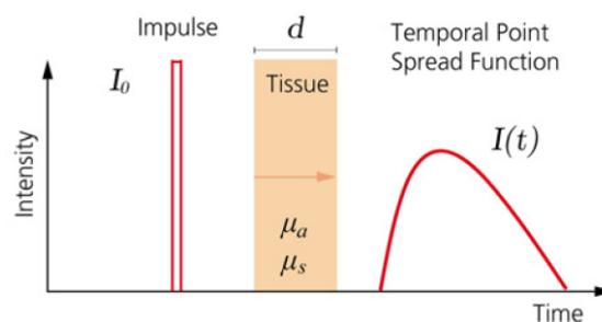
**Figure 2.6:** Time Domain NIRS principle, fig. taken from [11]
