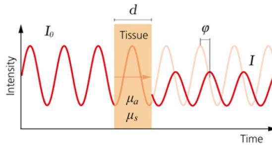
**Figure 2.5:** Frequency Domain NIRS principle, fig. taken from [11].
